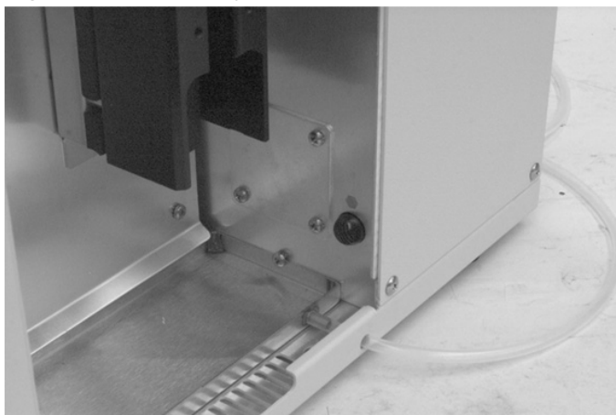
Figure 9. Drip tray with drain tube installed. Drain tube is positioned so tube can be visually inspected.
