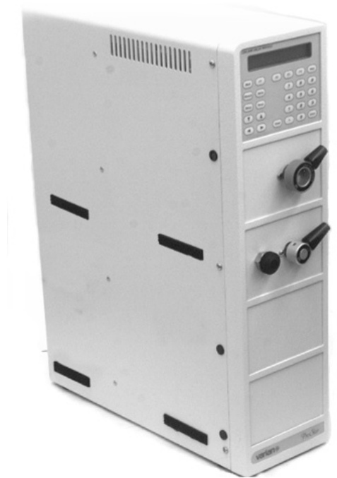
Figure 10. Example of positioning fabric strips on CVM for stabilization against a one- and two-LC module stack.
