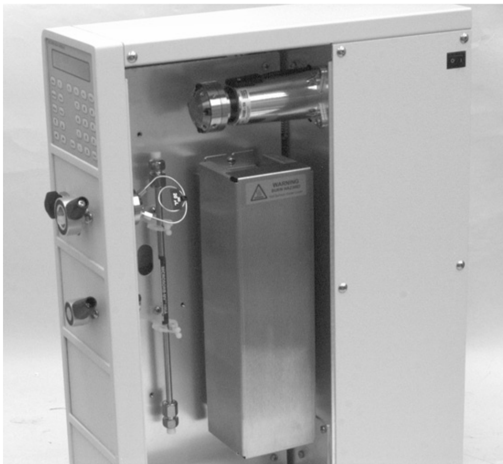
Figure 2. An example of an analytical-scale CVM configuration with one temperature zone and an automated, column-switching valve.
