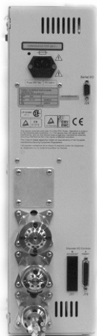
Figure 15. Rear view of a CVM, showing the power inlet, communication connections, and electrically actuated valves.
